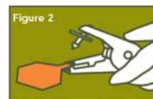
Slide button on pin. Tag and button are now ready for application.
